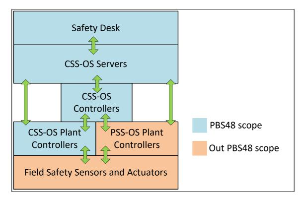
Figure 7-1 Standard Occupational Safety I&C conceptual architectures.
