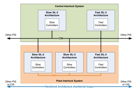
Figure 6-1: Standard Interlock I&C conceptual architecture.
