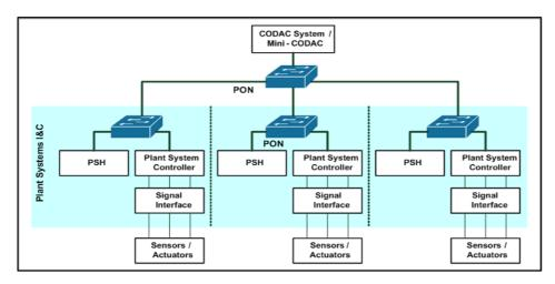
Figure 4-2: Plant systems I&C physical architecture - example 2, loosely coupled system. Plant system is decomposed in three plant systems I&C. Supervision is delegated to the CODAC system / Mini-CODAC.
