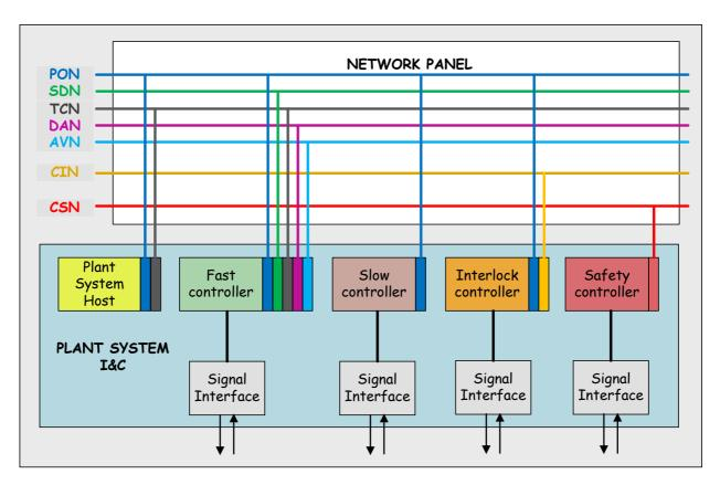
Figure 5-1: Network Interfaces between plant system I&C and Central I&C systems
