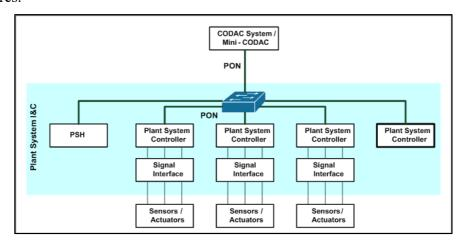
Figure 4-1: Plant system I&C physical architecture - example 1, tightly coupled system. Plant system has one supervising plant system controller (to the right). The supervising plant system controller coordinates three other plant system controllers which interface to the hardware.
